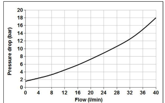
Pressure drop related to flow across reverse Check valve with throttle fully closed.
